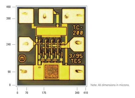
Figure 5. Bonding pad locations
