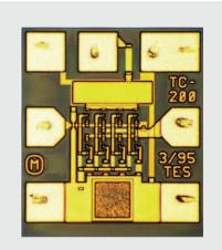
Chip Size:  $410 \times 460 \ \mu m \ (16.1 \times 18.1 \ mils)$  Chip Size Tolerance:  $\pm 10 \ \mu m \ (\pm 0.4 \ mils)$  Chip Thickness:  $127 \pm 15 \ \mu m \ (5 \pm 0.6 \ mils)$  RF Pad Dimensions:  $70 \times 70 \ \mu m \ (2.8 \times 2.8 \ mils)$  or larger
